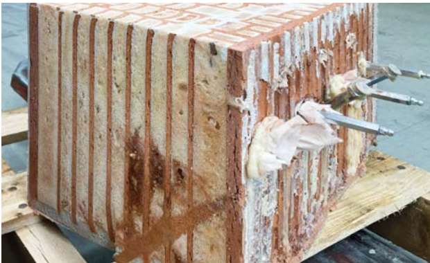
Fig. 3: Material filling (cross-section)
