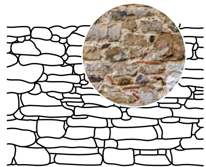
Quarry stone masonry
