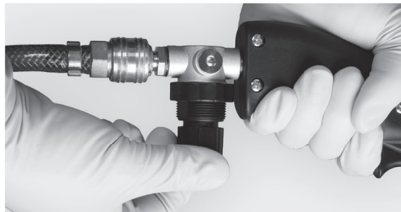
Connect the WEBAC® QuickSet Pump to the air compressor and adjust the feed pressure using the pressure control valve
