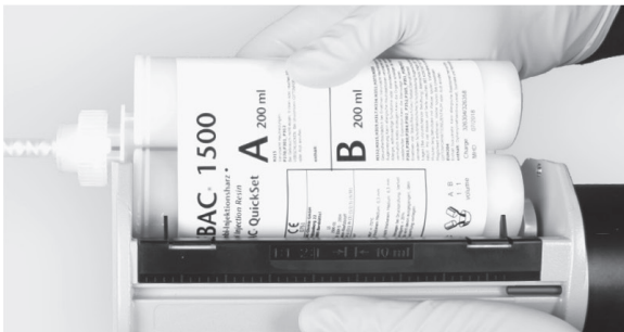
Check the mixing ratio of the insert tray and install the cartridge in the WEBAC® QuickSet Pump
