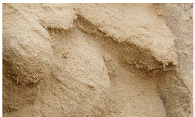
Fig. 6: Example of a gel curtain after injection
