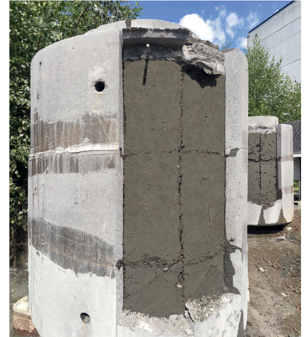
Annular gap filled with WEBAC® HIS (cut open for illustration)
